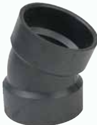
1/16 BEND ABS DWV SCHEDULE 40 22-1/2° ELBOW HUB X HUB
